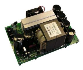
Fig. 3 4kW DC/DC boost converter developed in our laboratory
