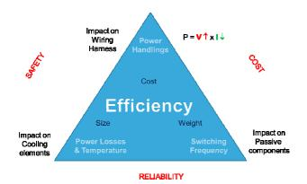
Fig. 1 Power semiconductor challenges for EV and HEV
