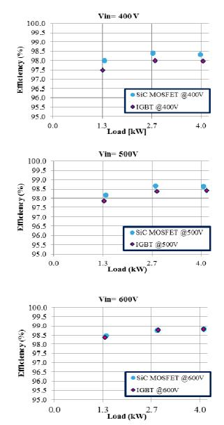
Fig. 5 Efficiency vs. load for input voltages Vin= 400 V, 500 V, 600 V
